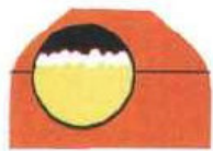
3 mixed with water and heated gradually to 76°C in the mash coppers.
