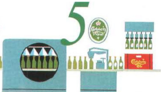
5 Finally, the pure, sparkling beer is brought to the high speed bottle-filling sections for automatic bottling, crowning, pasteurising, labelling and packing.
