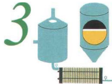
The wort is cooled in plate coolers and pure yeast is added. Fermentation takes place in vertical outdoor fermenting tanks. The yeast is removed and the beer matures in the tank for two to three weeks.
